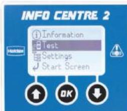
The **Test** menu displays data and operates some of the auxiliary functions of the EBS.
